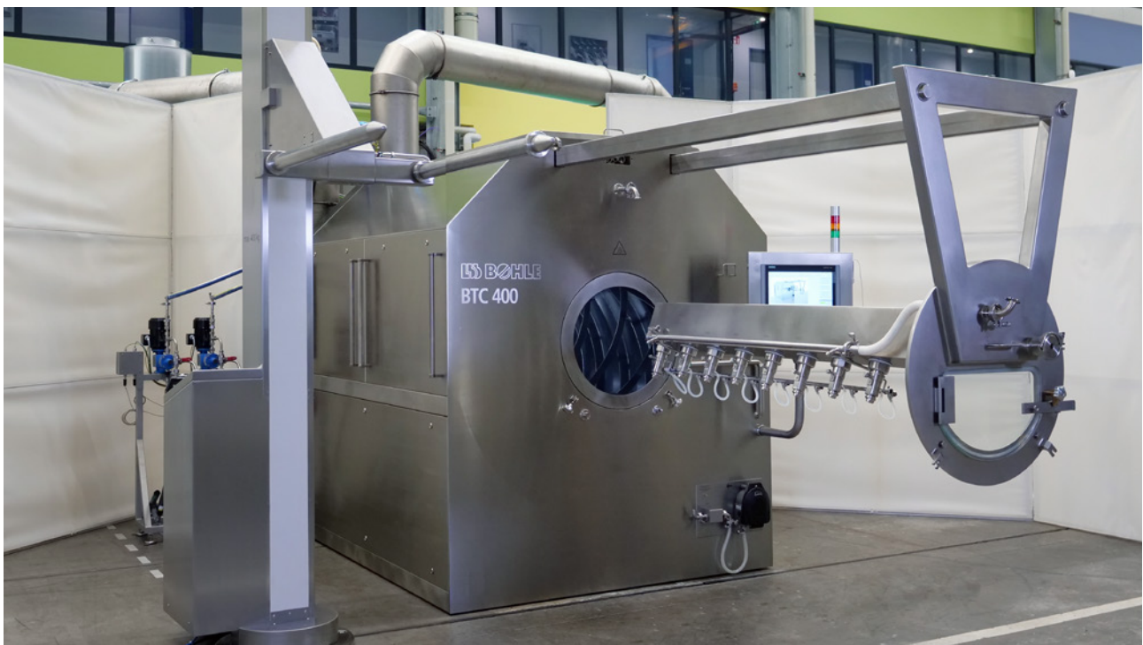
The BTC 400, here with lifting column of the SL series, enables up to 35% shorter process times compared to conventional coating systems.
